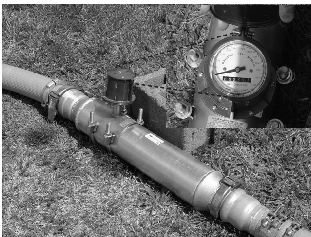
Figure 6. In-line flow meter with an exploded view of register
